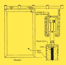
Available in Various Lead Values To Meet Individual Protective Requirements for Industrial Non-Destructive Testing or High Energy X-ray and Gamma Radiation Shielding Applications.
