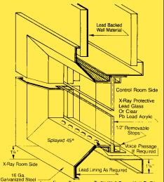
Inner Frame Telescopes To Fit Wall From 43/4" To 7 Rough Opening 1" Larger Than Glass Size On Control Side & 24" Larger On Splayed Side (2" Larger In Height For Frames With Voice Passage) • Frames also available in Stainless Steel or Aluminum
